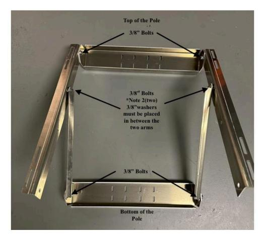
3.5. Attach the solar panel to the mount using the 1/4in hex bolts, washers, and nut and the 7/16 wrench. It is easiest to find a flat surface and lay the panel upside down and attach the solar arms as they rest on the panel. MAKE sure to have a flat surface or use the solar packing box so as to not crack the panel. Damaging a panel will result in an unusable system and will incur a replacement fee.
